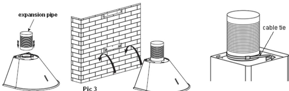
5. Fix the outside chimney bracket on the outside chimney and be sure that the inside chimney can be adjusted the height in it freely. Afterwards, install the chimney on the cooker hood and lift up expansion pipe till it out of the wall through the hole on the wall. See Pic 4.
