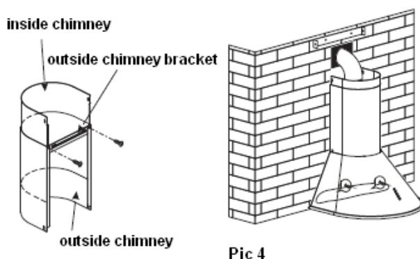
6. Adjust the height of the inside chimney to the position of the inside chimney bracket and fix on it with screws, meanwhile, fix the outside chimney on the cooker hood body by screws. After adjusting the position, fix the body with safety screws. Note: The two safety vents are positioned on the back housing, with a vdiiameter of 6mm. See Pic 5.
