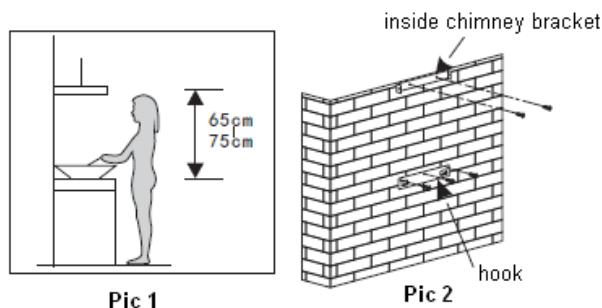
3. Install the hook on a suitable place once the installation height is fixed, and keep it in line. The fixed position of the inside chimney bracket is the place of chimney. See pic 2.
