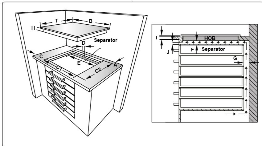
Apply the supplied one-sided self-adhesive sealing tape all the way around the lower edge of the cooktop. Do not stretch it.
